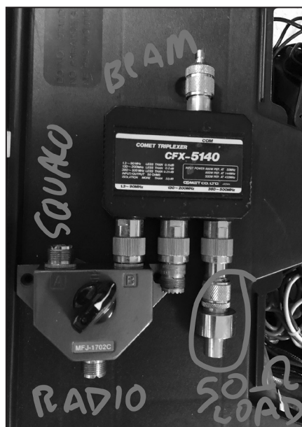
Figure 5 — Using a diplexer to improve band isolation.
